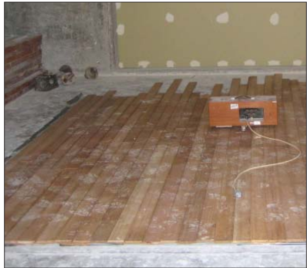
A test floor and 'tapping machine' at the CSIRO acoustic test laboratory in Melbourne
